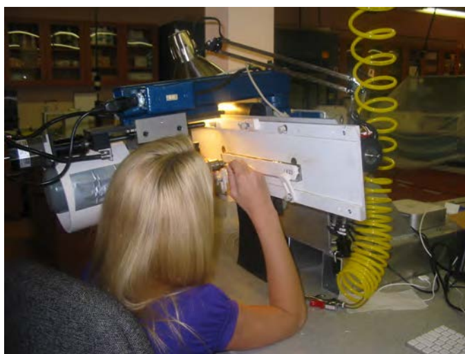
Figure 5. A chemist drills a slab of the coral Montastraea faveolata using a dental drill and collects the powder for Sr/Ca analysis. Photo credit: Jennifer A. Flannery, USGS.
